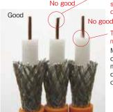
To make sure insulator part not remained on conductor
