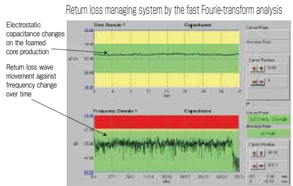
Sample : TCX-5CHD foamed insulator core production
